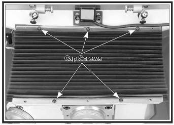
Figure 10. Front way cover installed.
